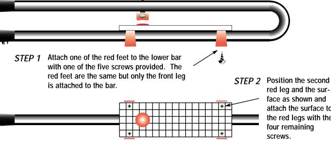
STEP 3 If your M-80 appears to be leaning to the left or right... loosen the screw that holds the front red leg to the bar... align the tube and tighten the screw.
