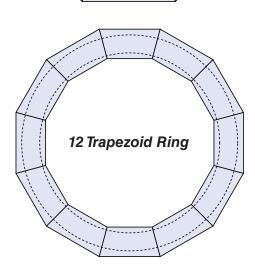
**12 Trapezoid Ring**... this option requires trapezoids that are made using a 75 degree angle setting on your Portable Glass Shop. This option will require more time to make. An example of how this might be appropriate is as a clock face using two different colors such as black and white in an art deco design.
