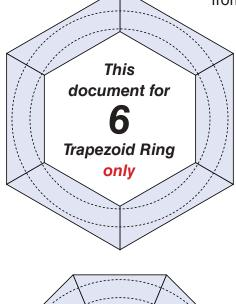
**6** *Trapezoid Ring*... this option requires trapezoids that are made using a 60 degree angle setting on your Portable Glass Shop. This option might be considered if your design is based on the hexagon. The disadvantage of this option is the length and width of the trapezoids needed.
