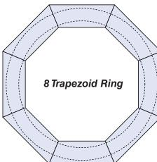
**8 Trapezoid Ring**... this option requires trapezoids that are made using a 67.5 degree angle setting on your Portable Glass Shop. This option might be considered if your design is based on the octagon. This option is usually preferred over the 6 trapezoid option because the strips needed to make the trapezoids are not as wide and yield less scrap.
