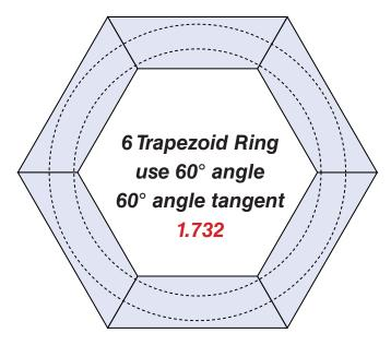
6 Trapezoid Strip Width Formula (base length - top length) ÷ 2 x 1.732 = strip width round up strip width to next millimeter if decimal greater than .3
